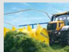
Grass Silage Spreader for silage clamps
