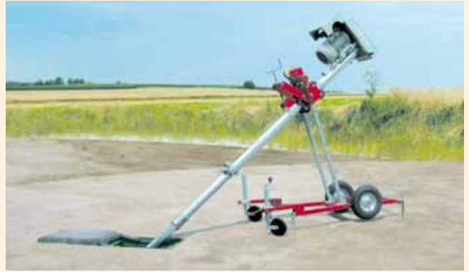
Type ETR - handy electric agitator with effective agitation performance, with winch and inclination adjustment. For tank openings from 0,60 m ø . Applicable until 5,0 m length of device and 11,0 kW (15 HP)
