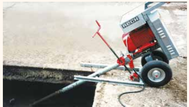
RECK electric channel mixer FUX with retain and inclination support (order code: EK-NB)
