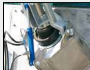
Rubber sleeve (second rubber sleeve inside for double safety optional)
