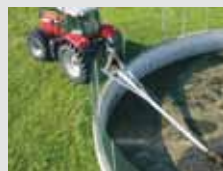
Slurry Mixer open slurry tanks and lagoons
