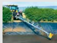
Slurry Mixer reinforced, for open slurry tanks and lagoons
