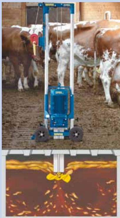
Folding propeller develops a sharp stream
