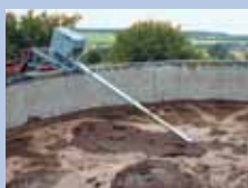
Electric slurry mixer for open slurry tanks and lagoons
