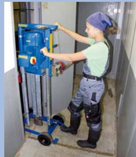
Advantage: Small turning radius in narrow corridors
