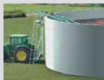
Tower Mixer for slurry towers up to an outside height of 6 m
