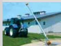
Slurry Mixer for covered slurry pits
