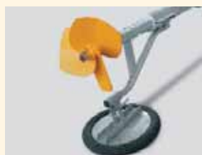
propeller stay with tyre fixation to protect the foil.
