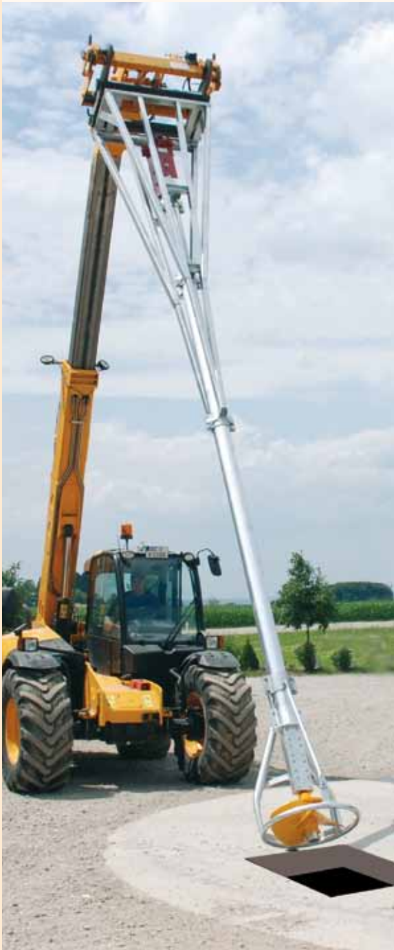
RECK hydraulic mixer TORANADO with telescopic loader and Euronorm quick coupling (order code: FHY)
