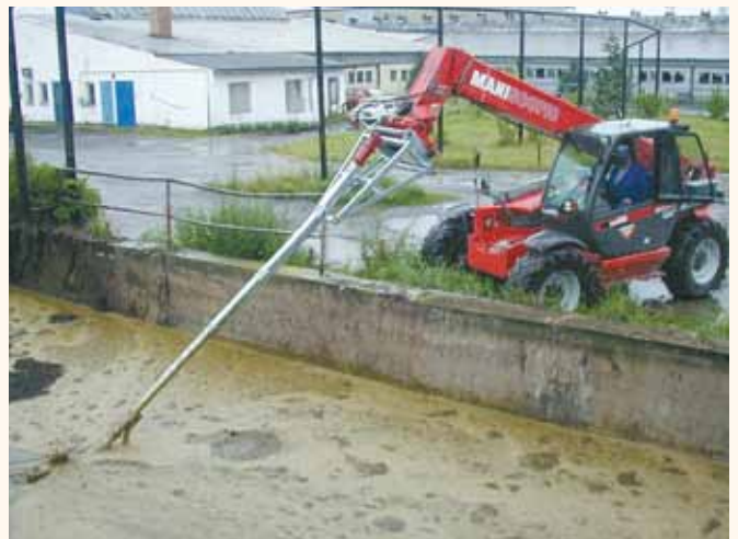
Special console with quick coupling for telescopic loader MANITOU.
