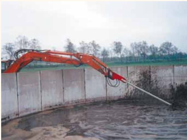
RECK Slurry mixer with hydraulic motor for effective mixing with the excavator boom.
