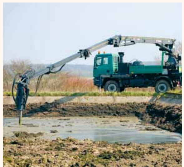
RECK slurry mixer with hydraulic motor TORNADO with crane boom for mobile use
