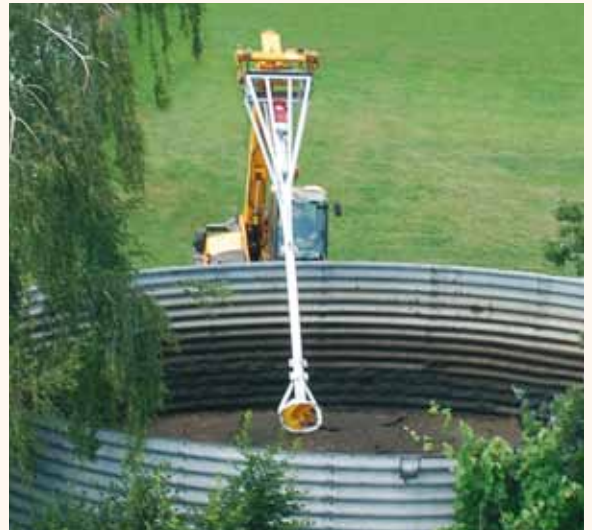
RECK slurry mixer with hydraulic motor TORNADO with telescopic loader in action at a slurry tower
